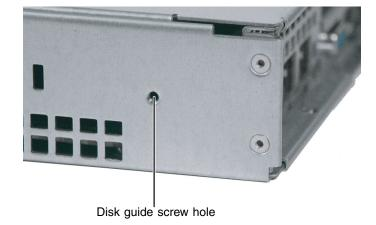
**4** Place a disk guide over the disk guide screw hole towards the back of the server.
